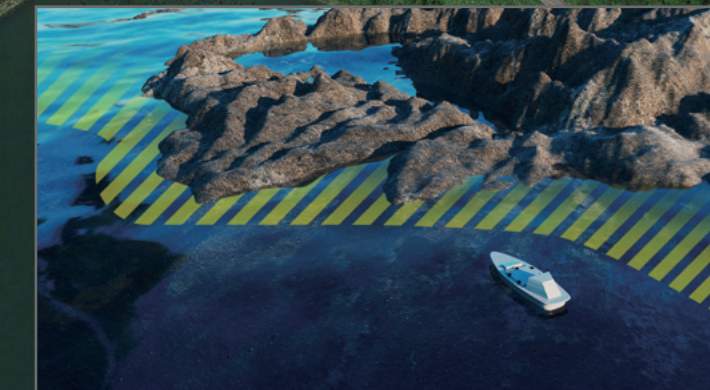
Boats equipped with multi-beam systems struggle to enter shallow waters
